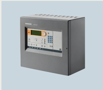
Fire control panel (1L, Comfort) FC361-ZA – Housing: 402x372x211 mm – Batteries: max. 2x 12 V, 25 Ah Order no.: S54433-C111-A1
